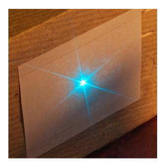
At this point you should have gotten the tube lasing on at least 514.5nm or 488.0nm. If you don't get the laser light flash, you may try some of the following:
