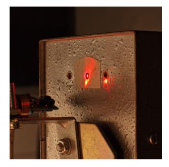
These reflections are from the OC and the HR, and should be made to converge with the central hole of the screen. The OC reflection may even be missing if the OC alignment is too far off. Adjust the OC first, and then the HR (prism), as precise as you can. The adjustment screws of the mirror platforms form a right angled triangle, avoid touching the screw at the vertex of the right angle, the other two should be used instead.
