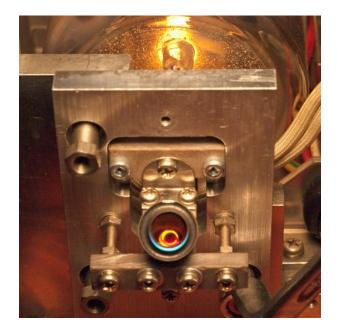
This offset will be taken into account when setting up the He-Ne laser, as will be described later. The adjustment screw in the top left corner of the mounting plate sets the prism pitch angle, and has the most effect on prism tuning for specific wavelengths.
